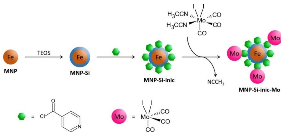
Fig. 1. Synthetic pathway adopted to prepare the MNPs.
